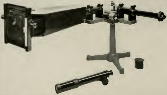
Fig. 9—Hilger wave-length spectrometer. The camera is interchangeably mounted with a reading telescope.
