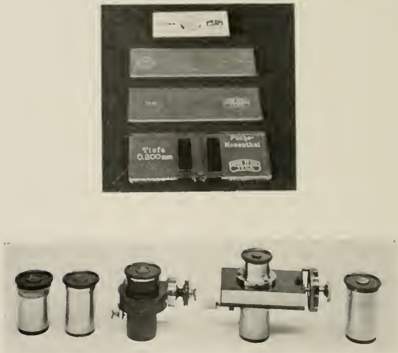
Fig. 26—Various types of eyepiece and stage micrometers used in connection with the microscope to obtain the dimensions of microscopic objects.
