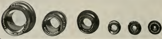
Fig. 4—A battery of low-power lenses. These lenses are used without eyepieces. Each lens is equipped with a diaphragm for stopping the aperture.
