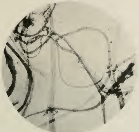
Fig. E. Paper fibers by 97 X. Note the surface markings; the gradation in color and the appearance of roundness possessed by some of the fibers. The photograph was taken with a modern medium-power apochromatic objective.
