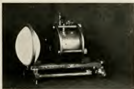
Fig. 2—Photograph of the Oscillator Used by Nichols and Tear. ( Physical Review )
