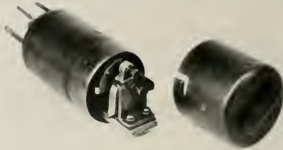
Fig. 7—Early supervisory relay
