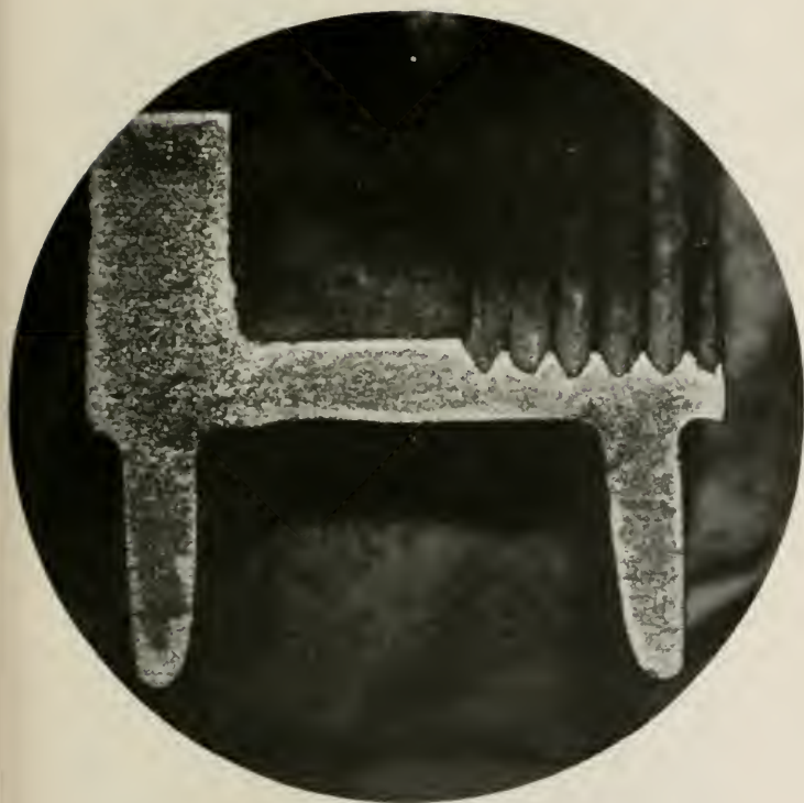
Fig. J. (a) Faulty pack hardening of car wheels for toll ticket distributing system. The object of pack hardening is to impart a highly carburized wearing surface to the otherwise soft steel part. The interior remains soft and ductile. Lack of uniformity in hardening or insufficient depth of the carburized zone causes soft spots which result in unequal wear. The magnification is 11.2 X.
