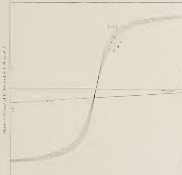
Fig. 7 Families showing relation between phase displacement and frequency for various power levels
