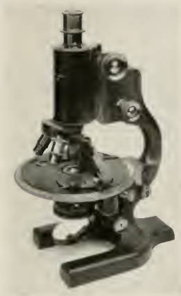
Fig. 3—Research type of microscope by Spencer Lens Co. Large barrel for photo-micrography; a large revolving stage with graduated circle, and a removable mechanical stage.
