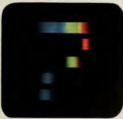
Fig. 10—Direct color photography of the spectrum of arc light and with the Wratten A, B, C and D filters respectively interposed in the beam.
