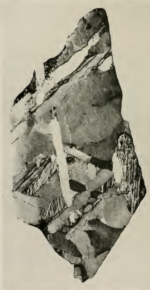
Fig. A. Meteoric iron consists of iron, nickel and the other elements usually found in steels such as carbon, sulphur, phosphorus, etc. The study of meteorites has contributed much valuable knowledge to the science of metallurgy. The Widmanstätten figures (shown by the arrangement of the constituents with reference to crystallographic planes) were generally considered characteristic of meteoric iron and it was believed that they were not to be found in manufactured iron and steel. Later this was shown to be an incorrect view.
