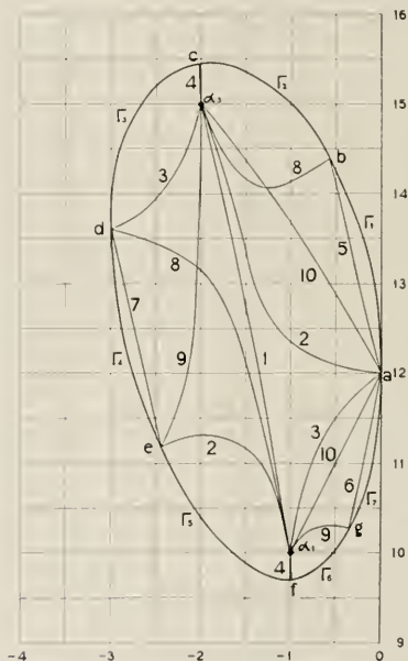
Fig. 4 -Domain of the poles of the driving-point impedance of a two-mesh circuit with two pairs of complex roots, showing the portions of the domain realizable by each network listed in Table III.
