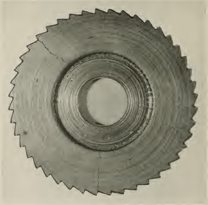
Fig. G. Season cracking of aluminum bronze ratchet wheels. (a) Ratchet wheel at magnification 2% X.
