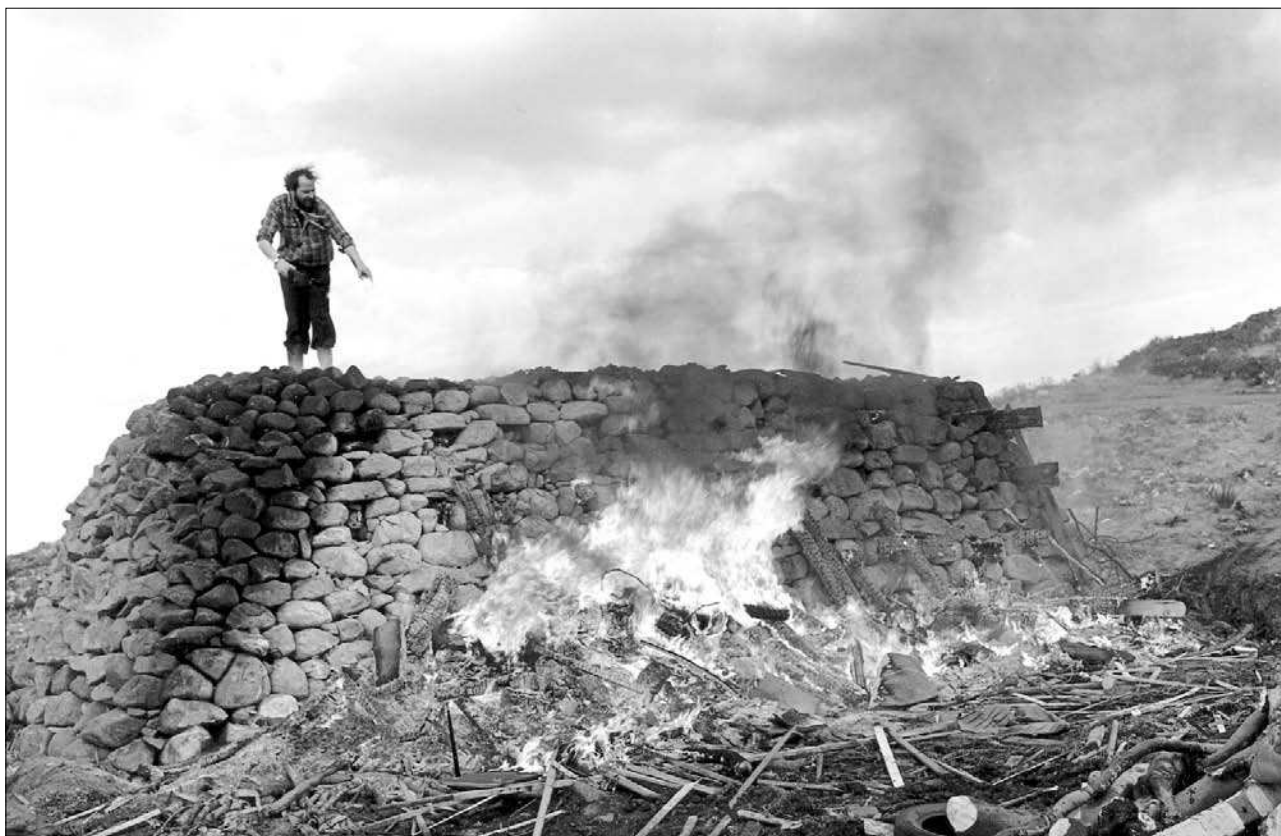
ILLUSTRATION 19.— Vitrified wall experiment at Aberdeen, 1980 (courtesy: James Livingston).
