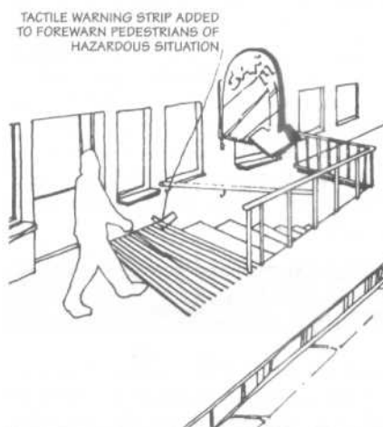
Figure 240-7. Unexpected level changes. Unexpected level changes are hazardous and should not occur in the main line of pedestrian walkways. Existing situations can be modified to forewarn unsuspecting pedestrians.
