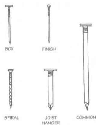
Figure 460-9. Nails commonly used in wood deck construction.
