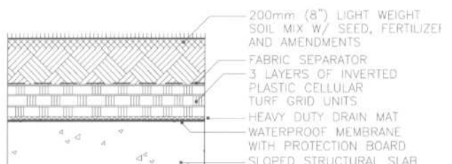
Figure 914-4. Natural turf athletic field- on structure. Fabric separator is required. A 300 mm (12") lightweight soil depth is preferred.
