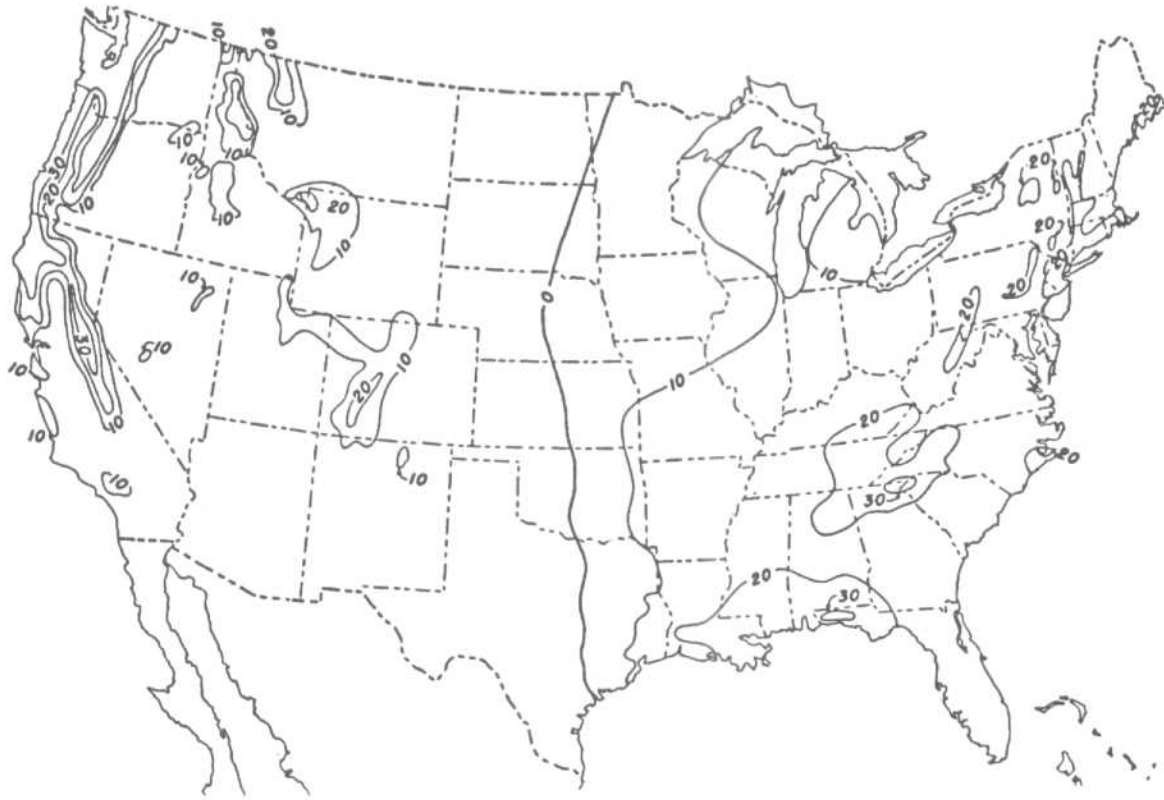
Figure 710-4. Areas of the United States where rainfall exceeds evapotranspiration (inches). Note that west of the zero line there is generally no annual excess except in mountain areas and in the Pacific Northwest.
