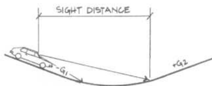
Figure 342-27. Headlight sight distance on sag vertical curve.
