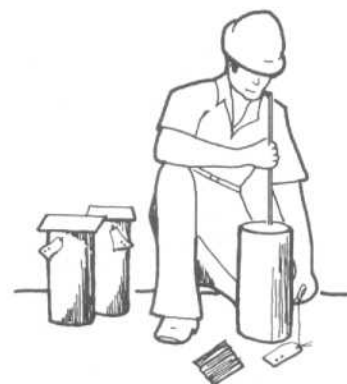
Figure 830-2. Cylinder test (ASTM C31). Cardboard or steel molds are filled with fresh concrete in three equal layers, and each layer is rodded 25 times with a \frac{5}{8} -in.-diameter tamping rod. Cylinders are lathed and covered with a plate or plastic bag.
