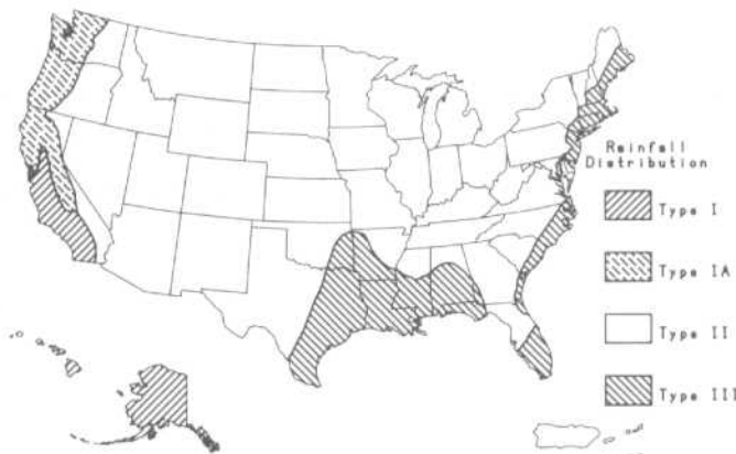
Figure 330-21. Map of approximate boundaries for SCS storm distribution types for the United States.
