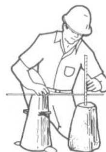
Figure 830-1. Slump test (ASTM C143). Slump cones are made of metal and are 12 in. high, with a 4-in.-diameter opening at the top and a 8-in.-diameter opening at the bottom. The cone is filled with concrete in three layers of equal volume, and each layer is rodded 25 times with a steel tamping rod. After the cone is filled and the top surface is smoothed, the slump cone is slowly lifted vertically and the subsidence (slump) is measured.
