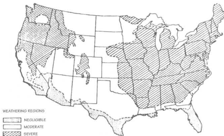
Figure 830-14. Weathering indexes in the United States. This index shows general areas where concrete is subject to severe, moderate, and negligible weathering. Data needed to determine the weathering index for any locality in the United States may be found or estimated from tables of local climatological data, published by the U.S. Weather Bureau, U.S. Department of Commerce, Washington, D.C.
