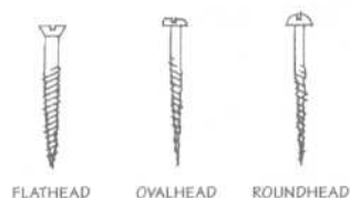
Figure 460-10. Wood screws commonly used in wood deck construction.
