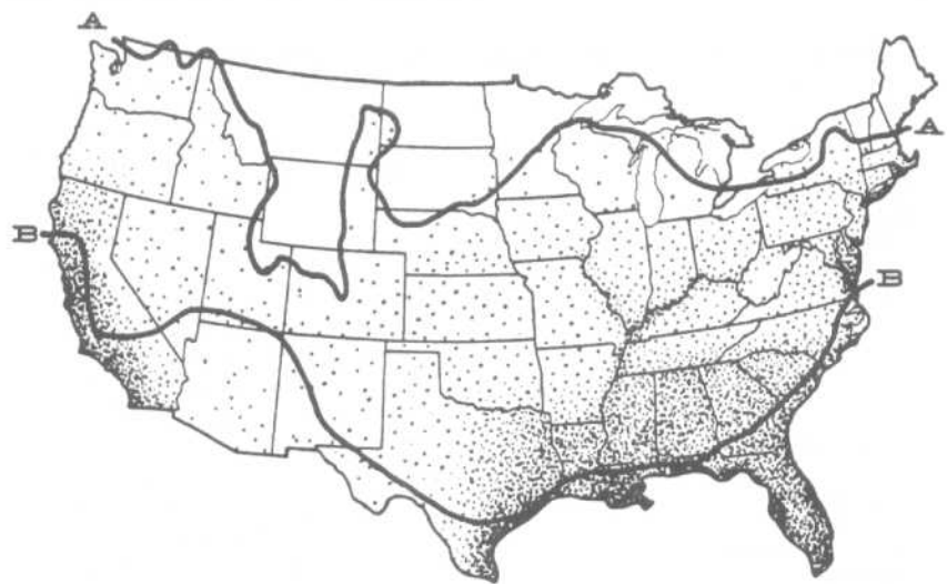
Figure 850-6. Extent of termite infestation in the United States. Zones illustrate general relative hazard of termite infestation. Subterranean termites have been found as far north as line A-A. Line B-B shows the northern limit of non-subterranean termites.
