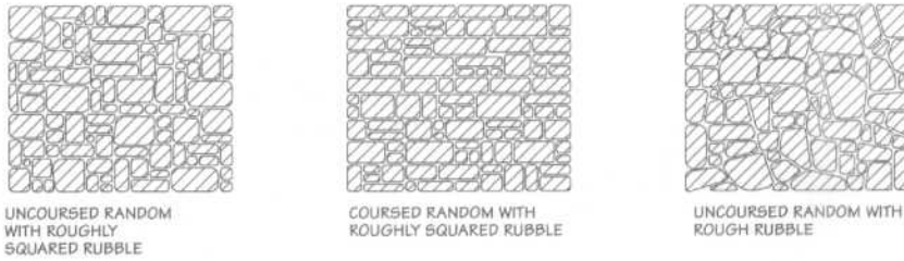
Figure 450-27. Random rubble masonry patterns. Units are squared and dressed by stone masons in the field.
